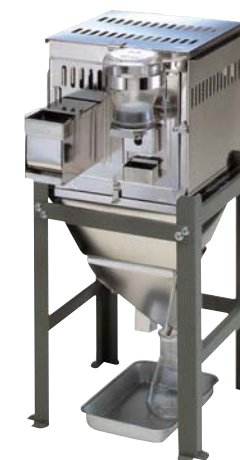
CL-0304 Rat Metabolic Cage (CT-10S) Type II Dimensions / 230×210×500mm Material / Stainless steel
